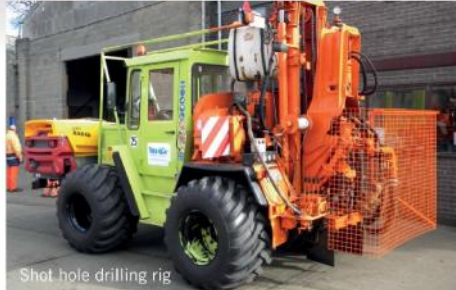
Shot hole drilling rig
